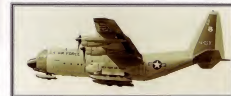
▼ Arctic operations Among the rarest of all Hercules were the ski-equipped C-130Ds flown by the New York Air National Guard. These aircraft were used to supply radar stations located in the Arctic.
